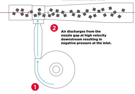
Turbo blower injects air into eductor venturi nozzle plenum.
