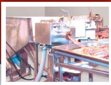
The casing removal system on the hot dog processing lines at Dietz & Watson's Philadelphia plant captures waste casings and steam from five peelers.
