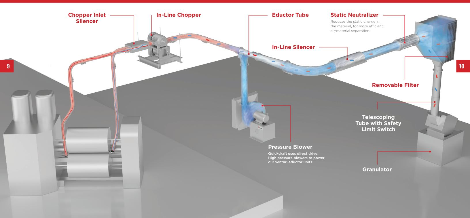
• Reliably convey challenging materials: static charge, abrasive materials, exposed adhesives,
